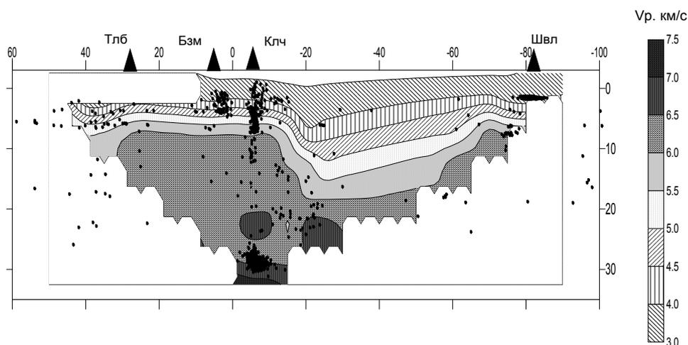
The velocity field is characterized by equal enough and quiet behavior of isolines. The isoline of 6.0 km/s velocity under volcanoes Klyuchevskoy and Bezymianny is fixed on depth of 8-10 km, at  $X = -20$  the km step-like immersing to depth of 18-20 km is observed, with the subsequent lifting in the direction of Sheveluch volcano.
