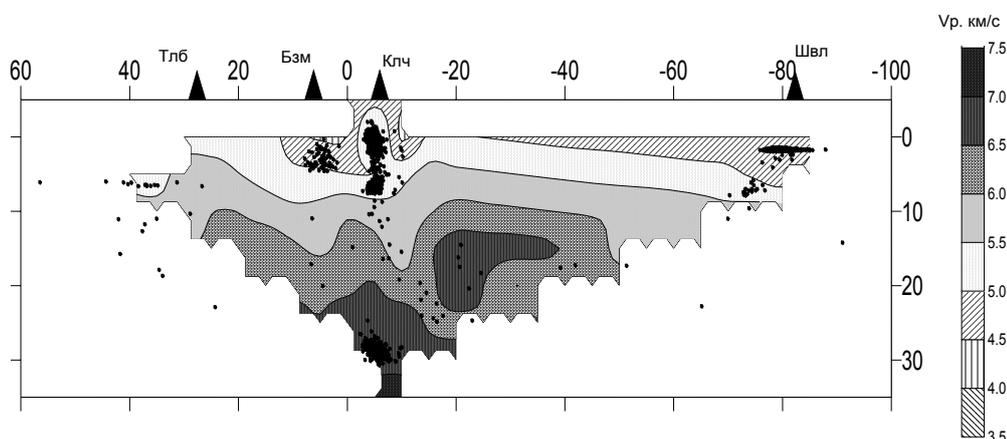
Character of the velocity has changed, perturbations in the form of ledges of isoline  $V_p=6.0$  km/s under the Klyuchevskoy volcano, and also an abnormal stain with values  $V_p=6.5-7.0$  km/s on depths of 15-20 km northeast of the Klyuchevskoy volcano are observed.
