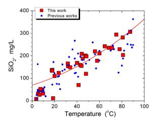
**Fig. 14.** Concentrations of dissolved Si expressed as  $SiO_2$  in Yurievskie waters vs outflow temperature. All data plot close to the solubility of amorphous  $SiO_2$  (log  $SiO_2 = 4.52-731/TK$ ; Fournier, 1977).
